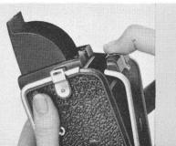
Turn the winding knob two or three turns to bind the end of the paper securely to the take-up spool. Be sure that the paper is started straight on the take-up spool.
